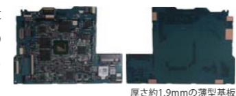
厚さ約1.9mmの薄型基板
