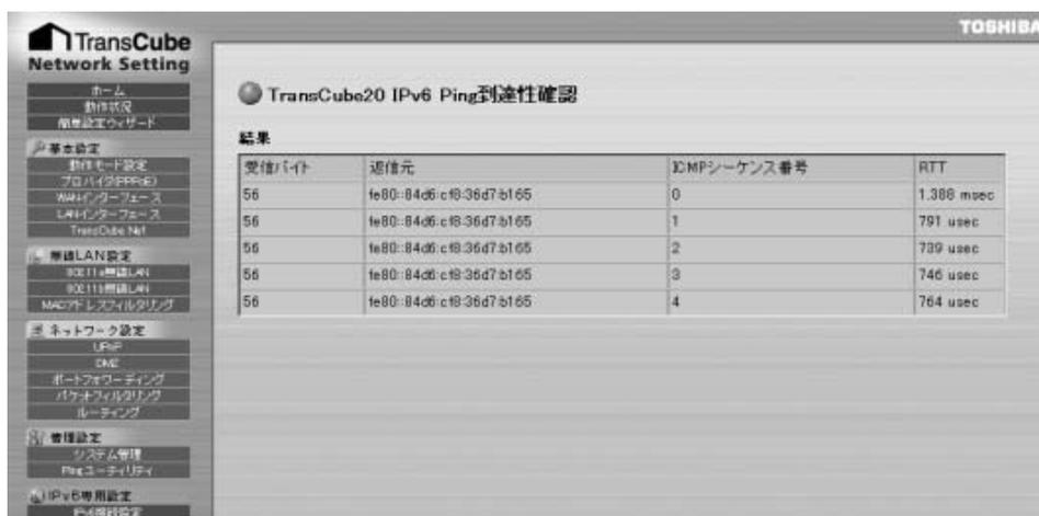
The screenshot shows the 'TransCube20 IPv6 Ping到達性確認' (TransCube20 IPv6 Ping Reachability Confirmation) page. It displays a table of test results with columns for '受信バイト' (Received Bytes), '返信元' (Reply Source), 'ICMPシーケンス番号' (ICMP Sequence Number), and 'RTT' (Round Trip Time).
