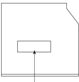
**CAUTION** CLASS 3B VISIBLE AND INVISIBLE LASER RADIATION WHEN OPEN, AVOID EXPOSURE TO THE BEAM.
